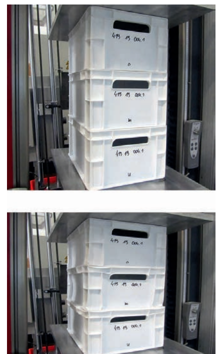
Fig. 3. Stacking pressure test with three stacked transport boxes with sandwich structure. Top: without pressure loading; bottom: strong pressure loading on the boxes visibly leads to a compression of the side walls and reinforcing ribs © TCKT – Transfercenter für Kunststofftechnik GmbH
