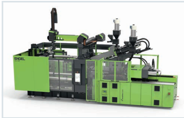
Fig. 1. In the Engel duo injection-molding machine equipped for the skinmelt process, the second plasticating unit for the skin material is mounted at a shallow angle above the horizontal injection unit for the recycled material
